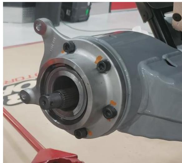
**28.** Install hub/rotor by aligning it with axle splines and pushing on until axle threads stick out. Put stock axle washer on axle and thread stock axle nut on over washer.
