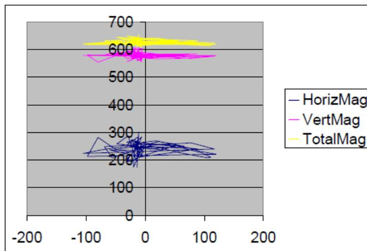
Figure 2 Magnetic field in earth frame versus heading with a carefully aligned magnetometer
