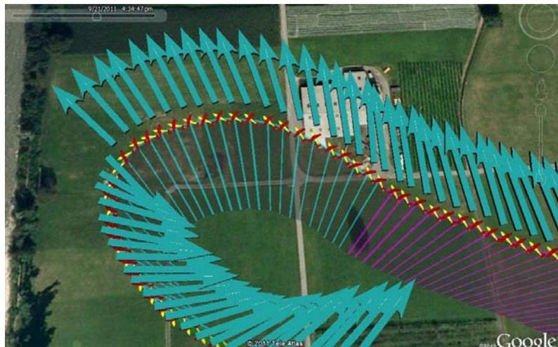
Figure 1 Apparent magnetic field reversal due to magnetometer misalignment
