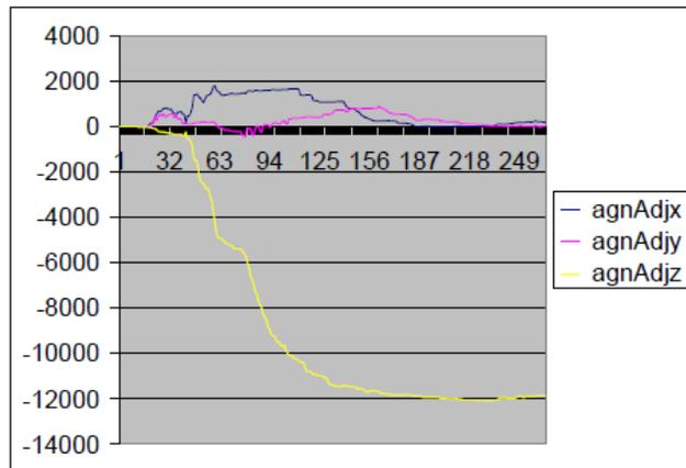
Figure 5 Convergence of realignment parameters for a 90 degree yaw misalignment
