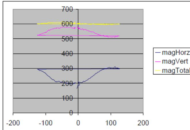
Figure 3 Impact of a 6 degree misalignment on estimated magnetic field versus heading
