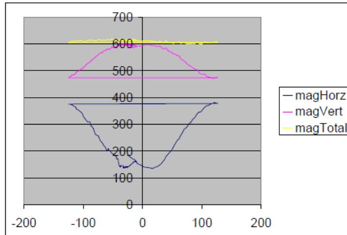
Figure 4 Impact of a 12 degree misalignment on estimated magnetic field versus heading
