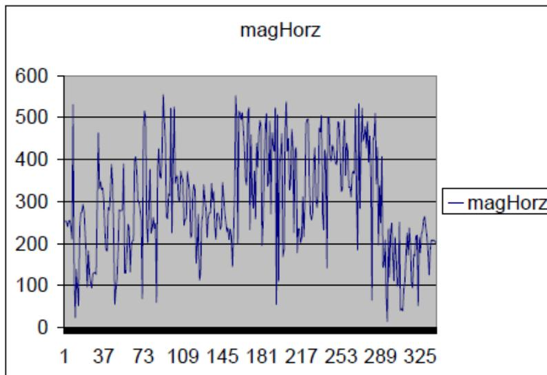
Figure 8 Horizontal component of magnetic field in earth frame with 180 degree yaw misalignment
