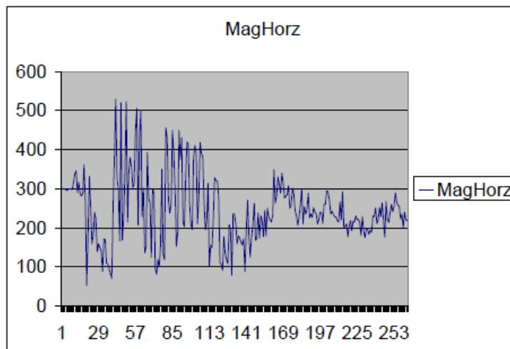
Figure 6 Horizontal magnetic field in earth frame with 90 degree yaw misalignment
