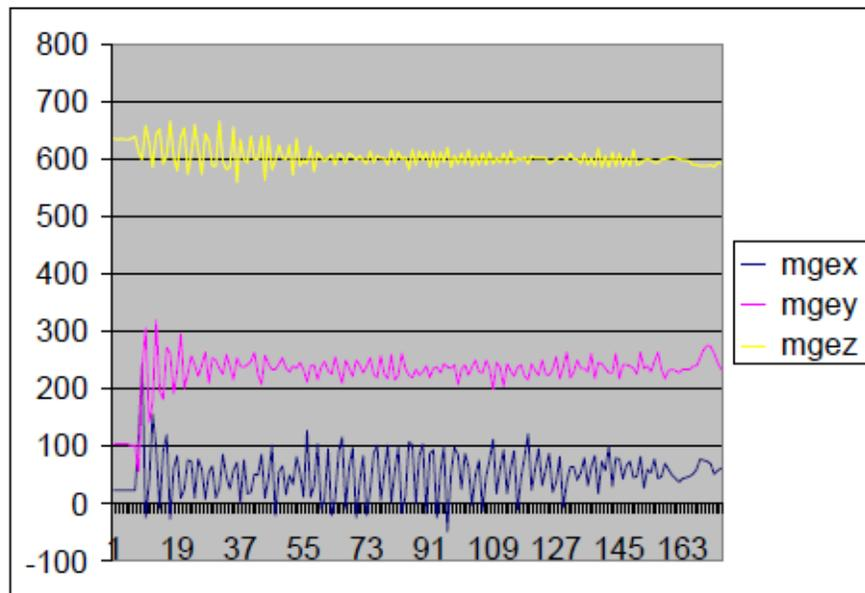
Figure 9 Plot of the X, Y, and Z component of the measured magnetic field in the earth frame, during an extended spin test at 78 RPM
