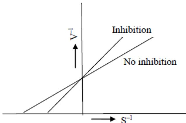
The nature of inhibition shown in the plot is
